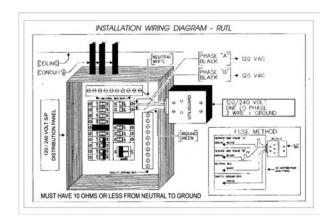
NOTE: When installing, keep the power leads, and neutral lead (or white wire) from the UtiliGuard® no longer than 24 inches in length from the connection point on the electrical panel. If the leads have to be longer than 24 inches, keep the leads at 24 inches, and splice in 6-gauge wire (of the same type and rating) for the required remaining length. (Ilsco SPA-2 in-line splice/reducer recommended, but any mechanical in-line butt splice will be acceptable.) DO NOT USE WIRE NUTS!!!
